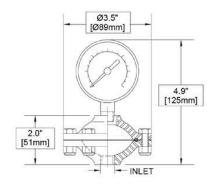
Housing: 316L Stainless Steel Alloy 20 <u>Diaphragm:</u> EPDM PTFE Viton
