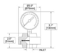
Housing: CPVC PVC Polypropylene PVDF <u>Diaphragm:</u> EPDM PTFE Viton Inlet Size: Up to 0.75"
